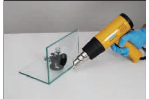
Third, completely dry edges to be bonded with Hot Air Heat Gun Cat. No's LD121 or UV8978
